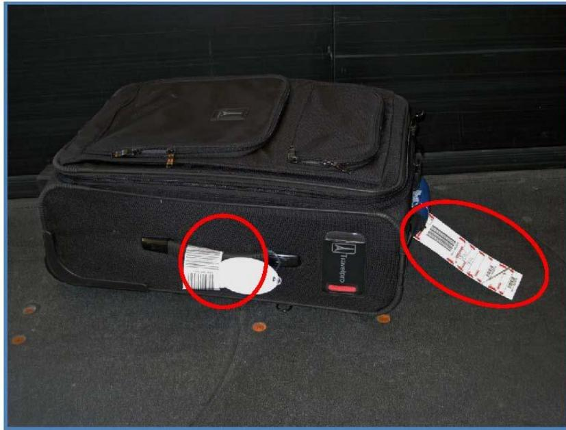
Photo 1 – “Unrecognized Tag” caused by multiple barcodes.
