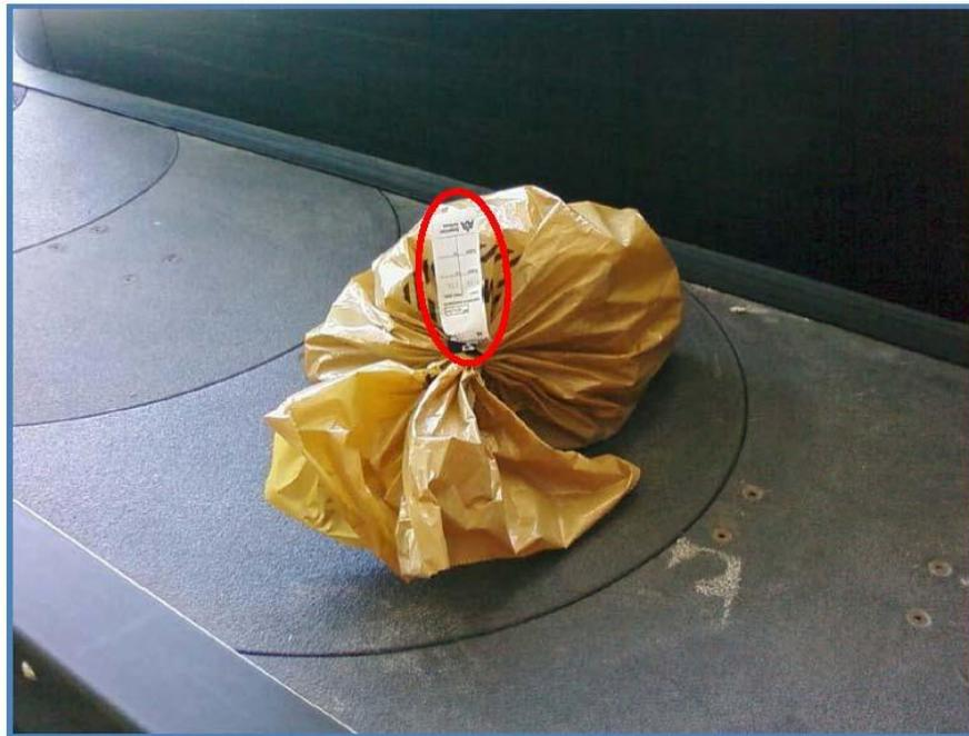
Photo 4 – “No Read” caused by COMAIL barcode not fitting sort parameters and unreadable barcode.
