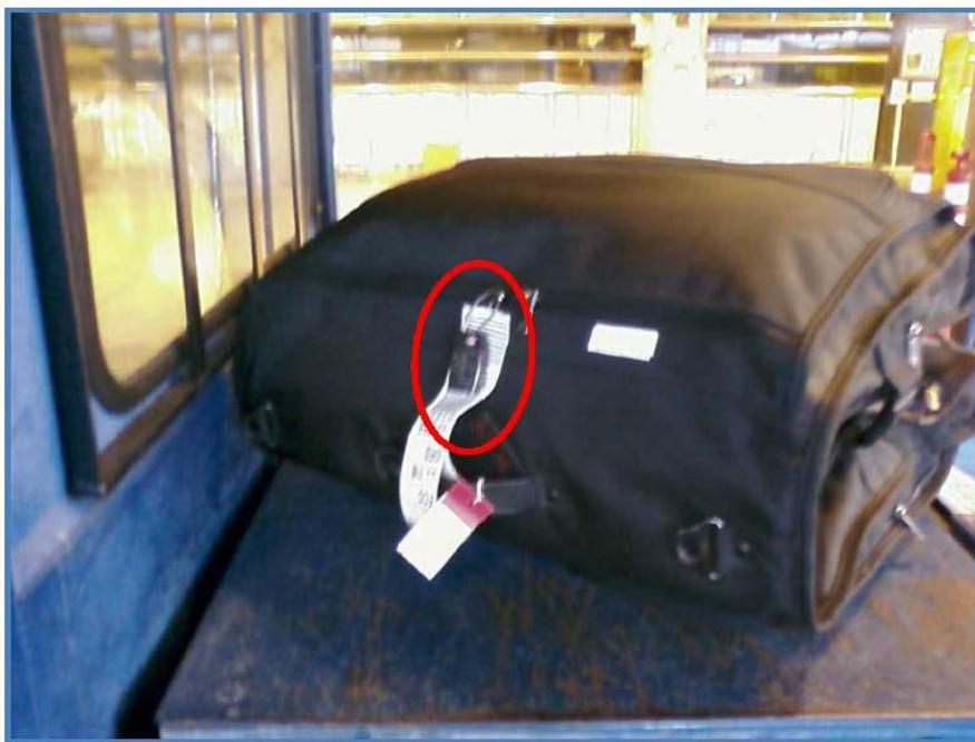
Photo 8 – “No Read” caused by barcode being blocked by object on bag.
