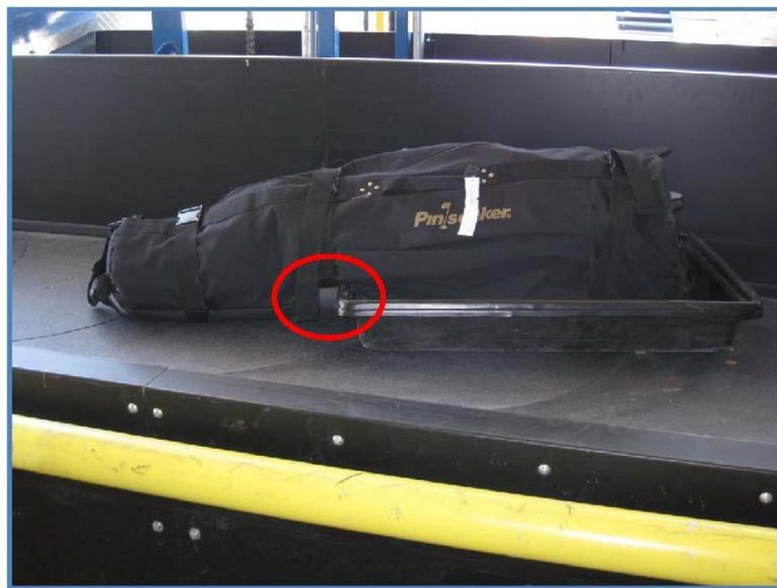
Photo 2 – “Jam” caused by one bag being detected as two as a result of gap under bag.
