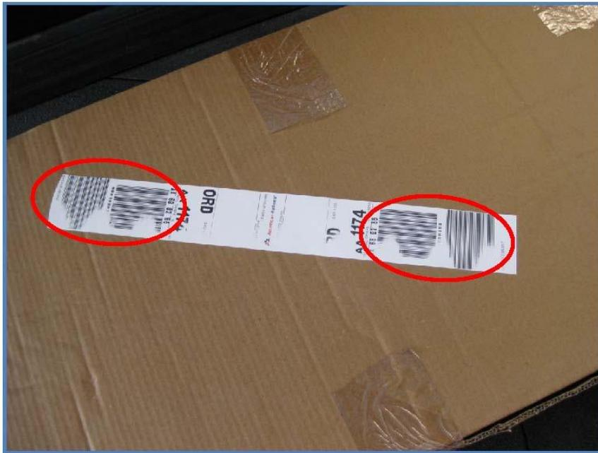
Photo 5 – “No Read” caused by poor tag print quality.
