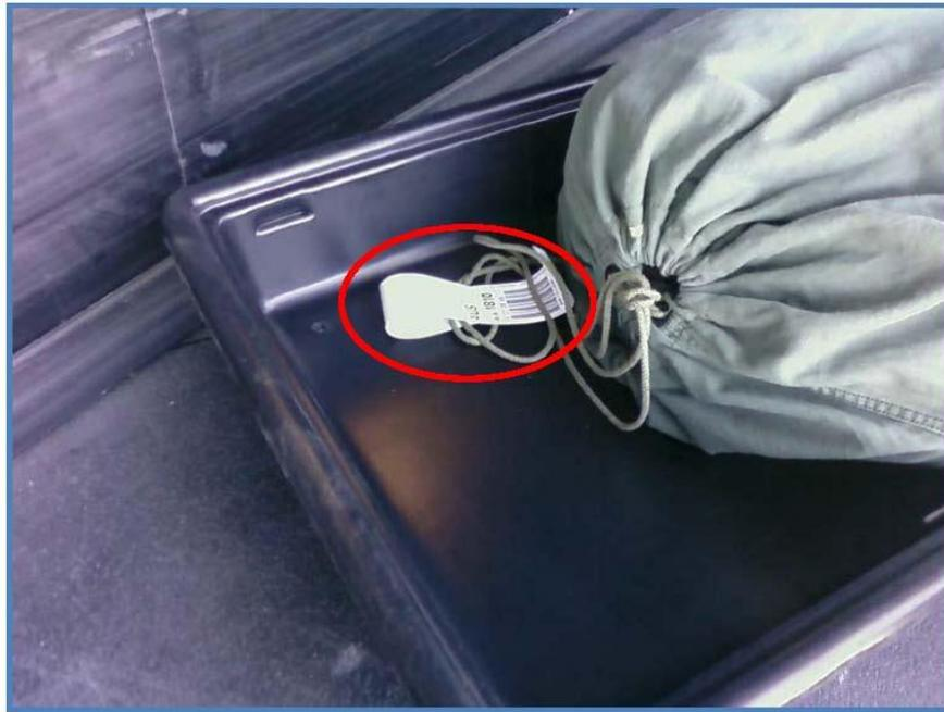
Photo 3 – “No Read” caused by poor barcode presentation and partially blocked barcode.
